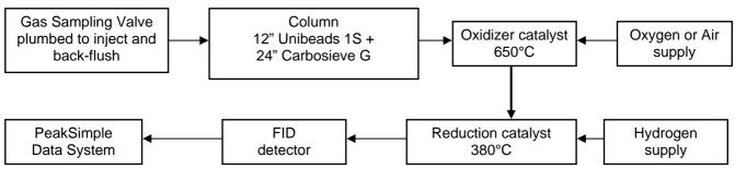
A typical calibration standard chromatogram is shown at right. The gas sampling valve backflushes all hydrocarbons into the catalysts and FID detector after the CO2 peak. Because all peaks are converted to methane, the back-flush peak represents the true carbon content of all the various hydrocarbons in the back-flush.
